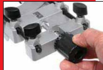
**Adjusting the fence using the microfence adjuster.**
