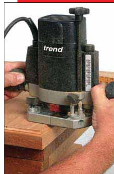
**Edge profiling with a bearing guided ogee cutter Ref. 46/30X1/4TC.**
