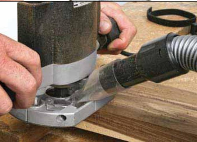
50mm plunge action is smooth and accurate and quickly locks with the now wonderfully comfortable side handles! The benefits of all the extra power soon become clear with the bigger cutters and you can now make a reduced number of passes, the full wave electronics maintaining a constant speed even under load. Where you
