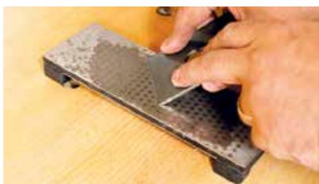
▲ Used with the bench stone the rubber construction keeps everything secure to the bench
